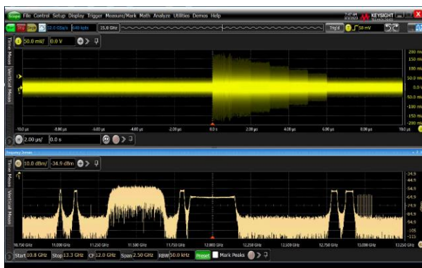
Figure 7. M9484C VXG RF output of 6 pulse-on-pulse scenario with comms interferers
