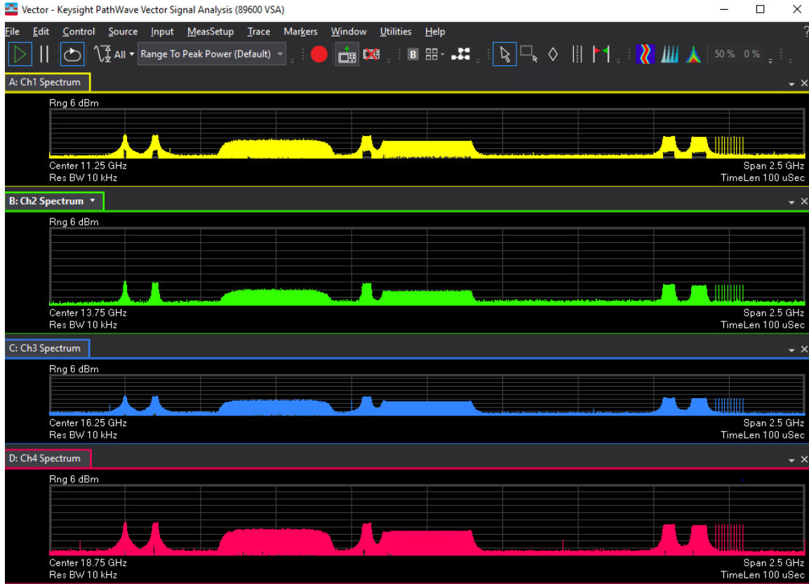
Figure 5. Example scenario with 8 different signal types including pulsed emitters, communication interferes, etc. duplicated across 4 M9484C VXG RF output ports all independently tuned.
